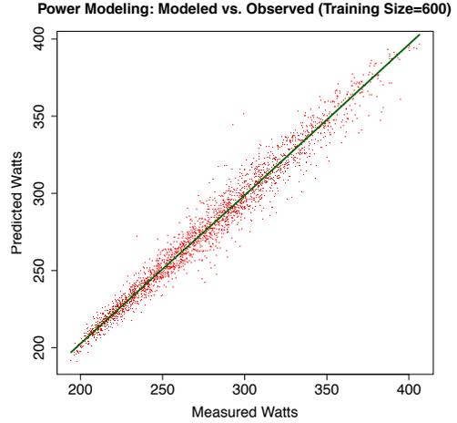
Fig. 2. Modeled vs. Observed Total System Power Draw
