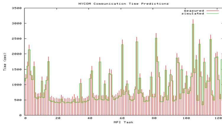
**Figure 5. Measured and simulated communication times for all tasks.**
